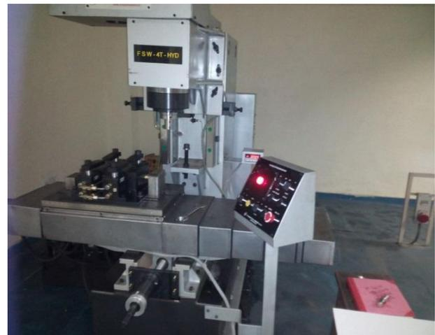
Figure 1: Friction stir welding / processing machine (DTU)
