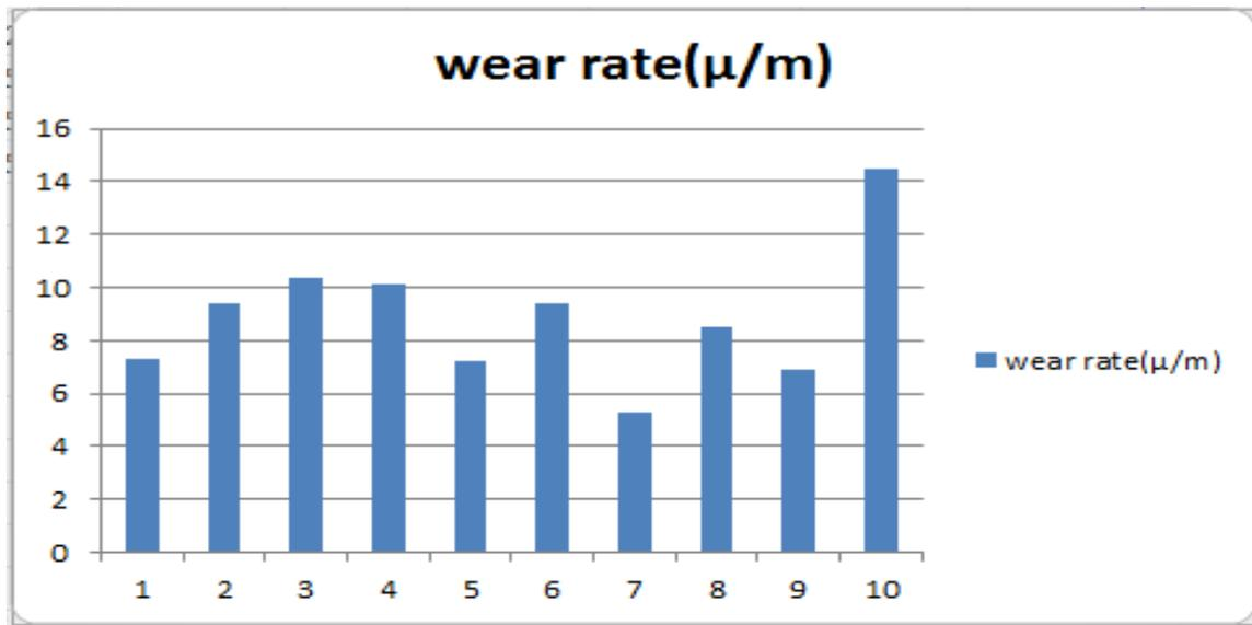
Figure.5: Wear rate in microns per meter sliding distance for each specimen
