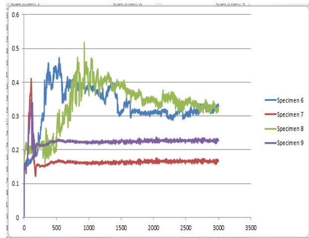
Figure.7: Friction coefficient vs sliding distance for various specimens
